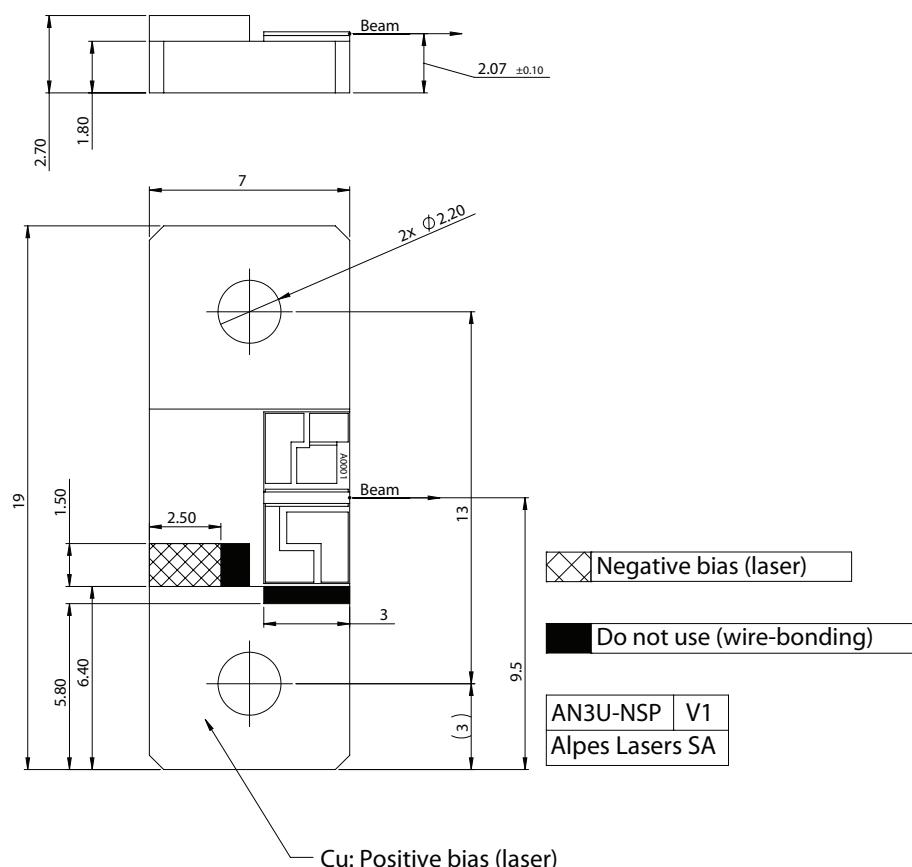
Figure 1: Mechanical and electrical interface for #sbcw10186 DN
