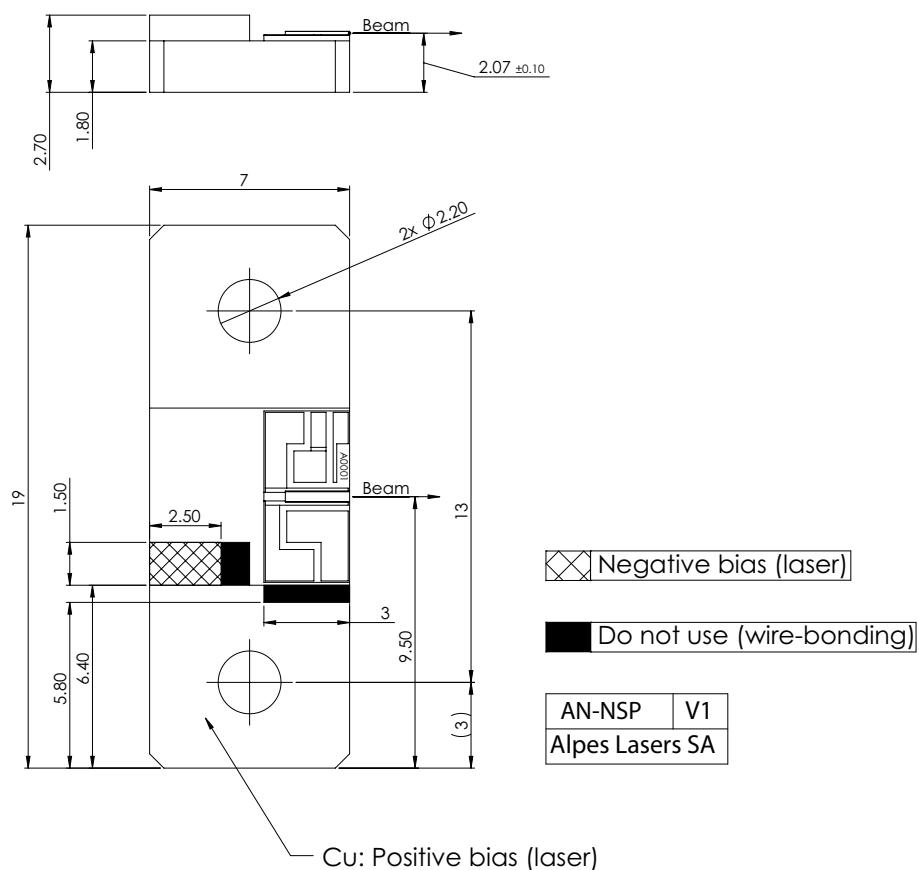
Figure 1: Mechanical and electrical interface for #sbcw10334 DN
