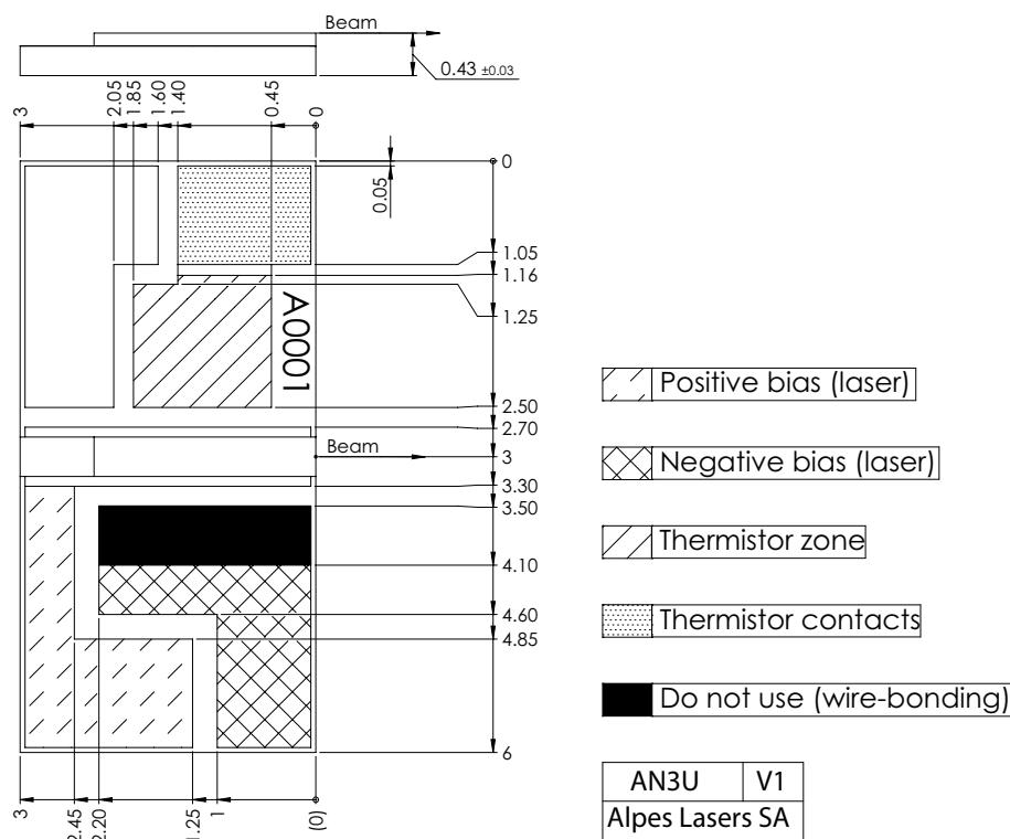
Figure 1: Support mounting for #sbcw10408 DN (please note that AlN submount numbering is A03AX)
