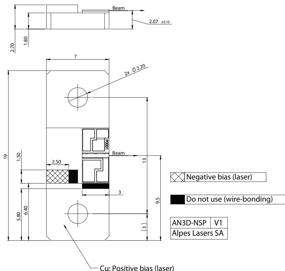
Figure 1: Mechanical and electrical interface for #sbcw12301 DN
