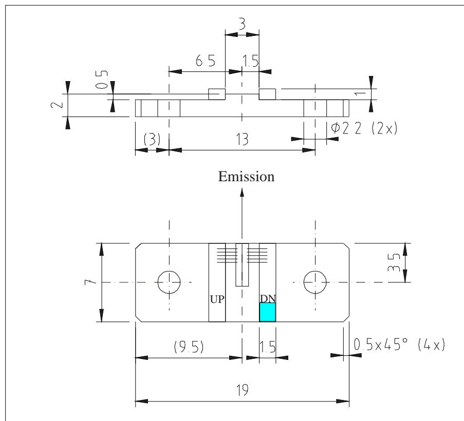
Figure 1: Support mounting for #sbcw1247 DN (please note that the laser is connected to the DN pad drawn in blue)
