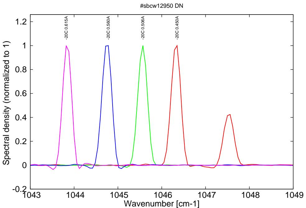
Figure 6: spectra at -20C for various DC currents (bimode at threshold, then becomes monomode)
