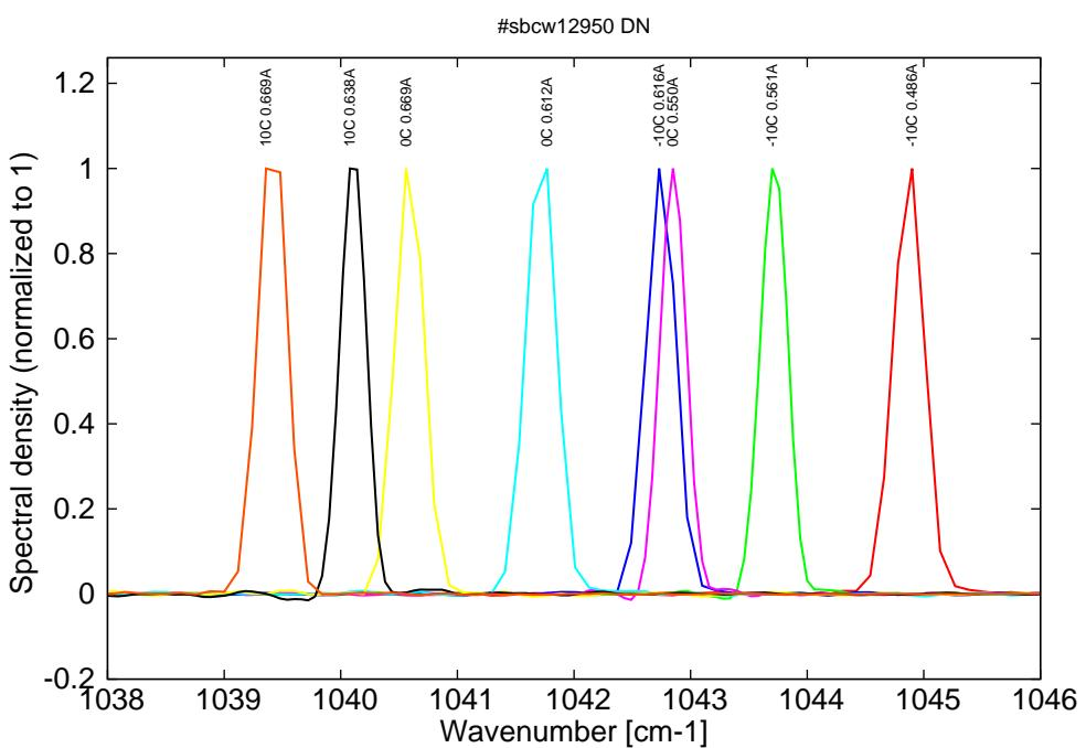
Figure 7: spectra between -10C and 10C for various DC currents (all monomode)
