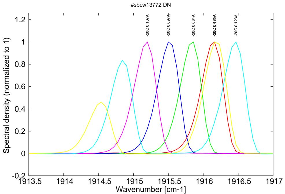
Figure 6: spectra at -20C for various DC currents (monomode up to 0.105A, then becomes bimode)
