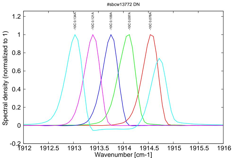
Figure 8: spectra at -10C for various DC currents (monomode up to 0.12A, then becomes bimode)
