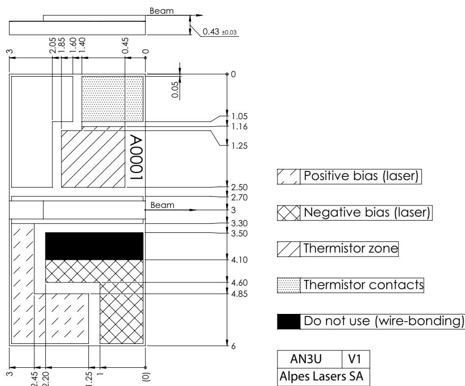
Figure 1: Mechanical and electrical interface for #sbcw13828 DN (please note that AlN submount numbering is A0GRE)
