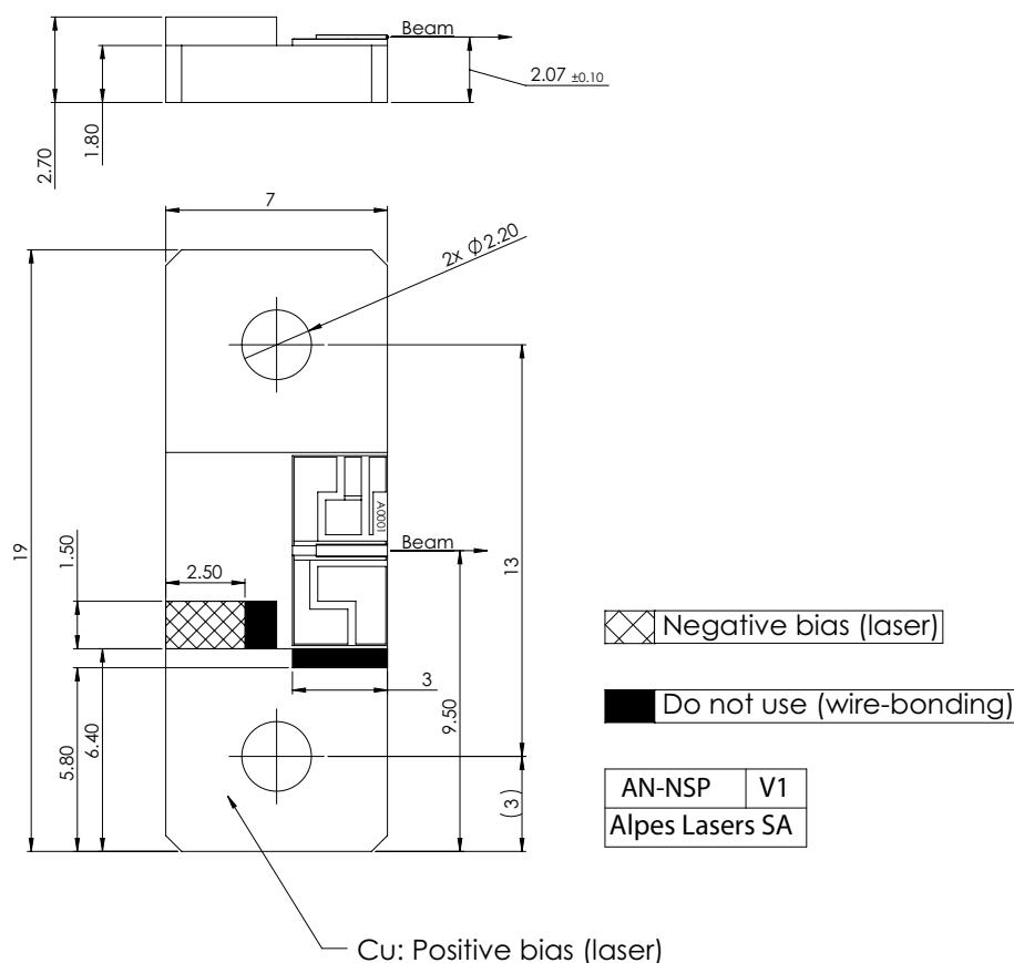
Figure 1: Mechanical and electrical interface for #sbcw13866 DN
