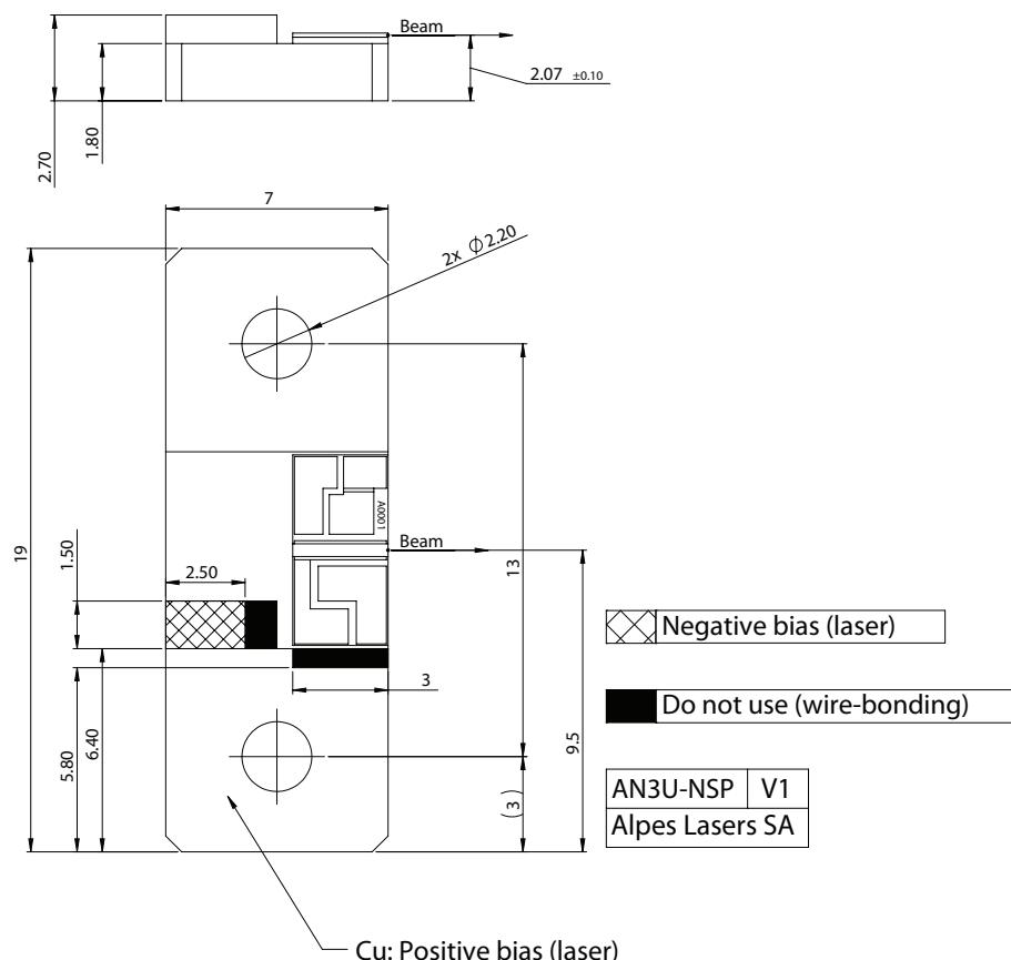
Figure 1: Mechanical and electrical interface for #sbcw14374 DN
