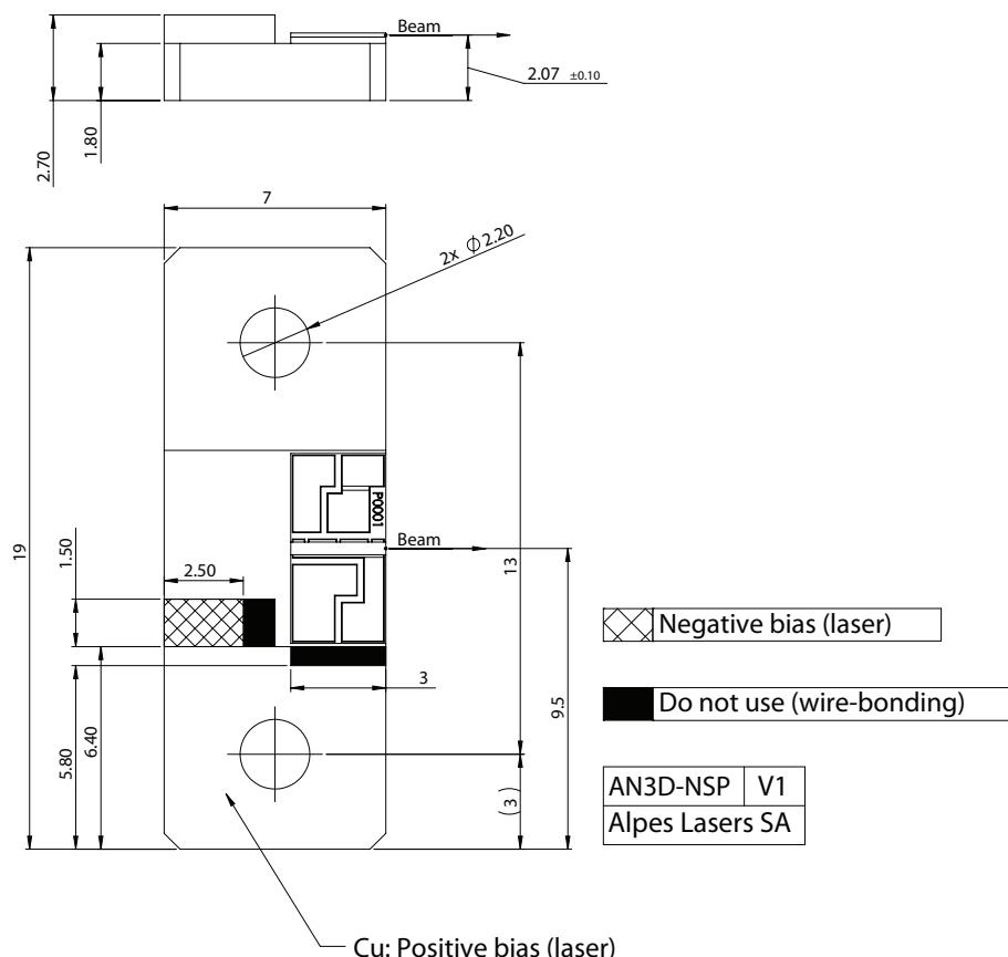
Figure 1: Mechanical and electrical interface for #sbcw14534 DN
