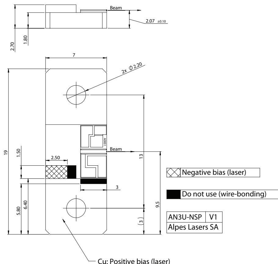
Figure 1: Mechanical and electrical interface for #sbcw15381 DN
