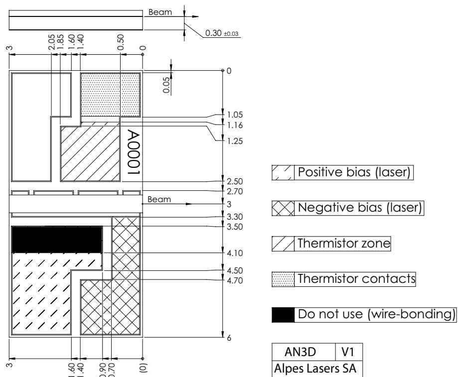
Figure 1: Mechanical and electrical interface for #sbcw15509 DN (please note that AlN submount numbering is P0988)
