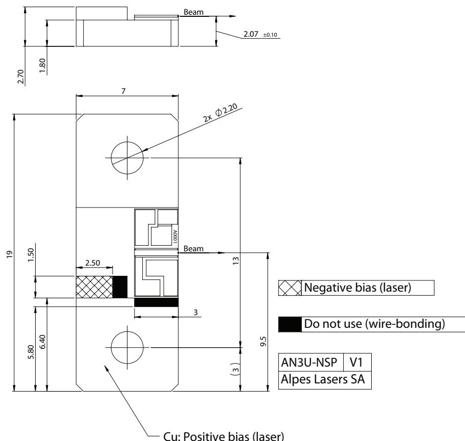
Figure 1: Mechanical and electrical interface for #sbcw16410 DN
