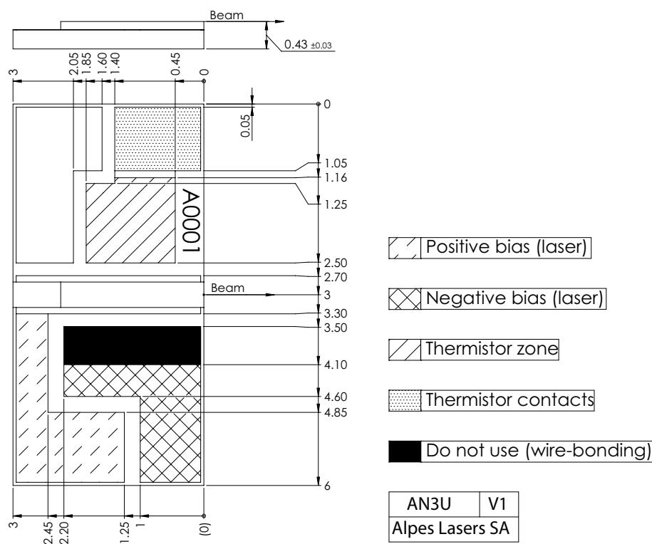
Figure 1: Mechanical and electrical interface for #sbcw17435 DN (please note that AlN submount numbering is A0M02)
