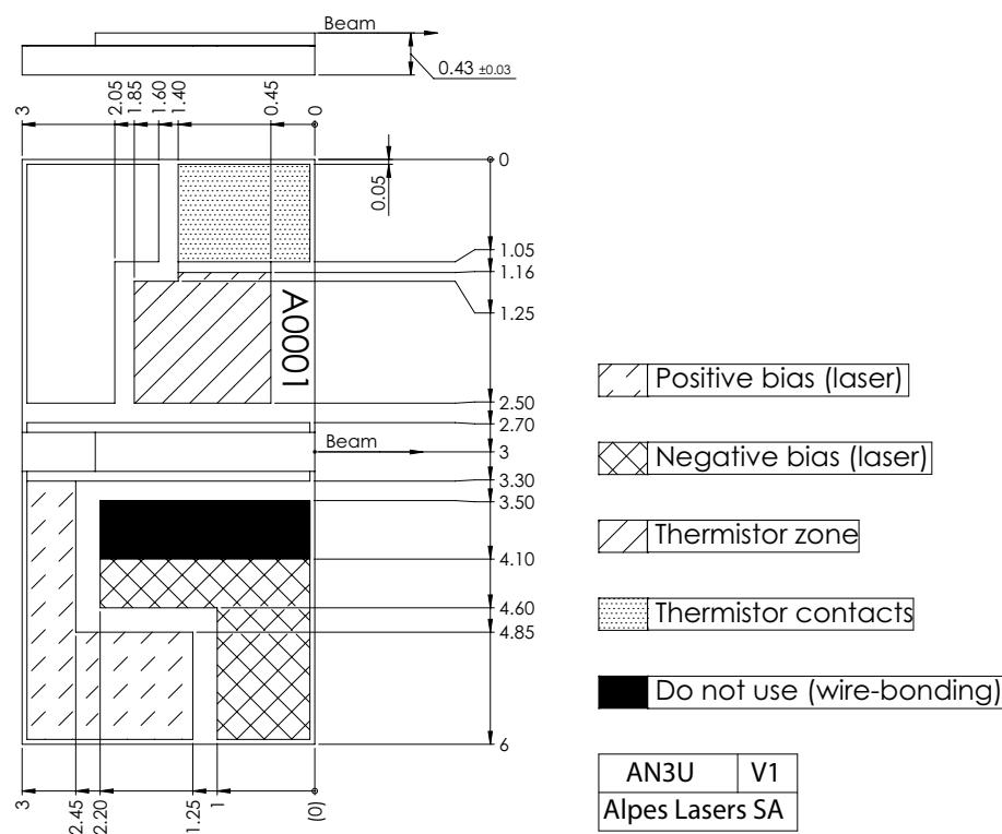
Figure 1: Mechanical and electrical interface for #sbcw17549 DN (please note that AlN submount numbering is A0L0R)
