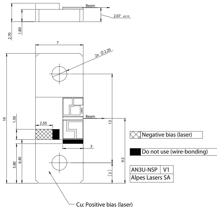
Figure 1: Mechanical and electrical interface for #sbcw18570 DN
