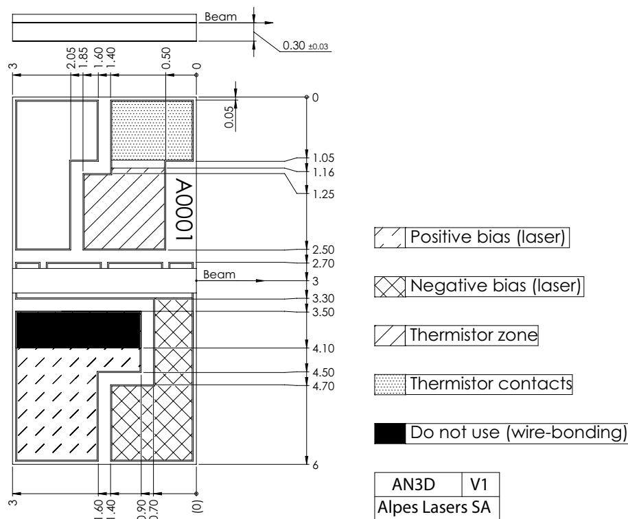
Figure 1: Mechanical and electrical interface for #sbcw19521 DN (please note that AlN submount numbering is P1134)
