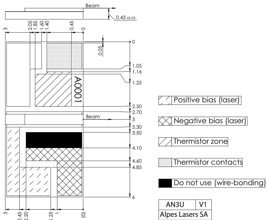
Figure 1: Mechanical and electrical interface for #sbcw19779 DN (please note that AlN submount numbering is A0PC3)
