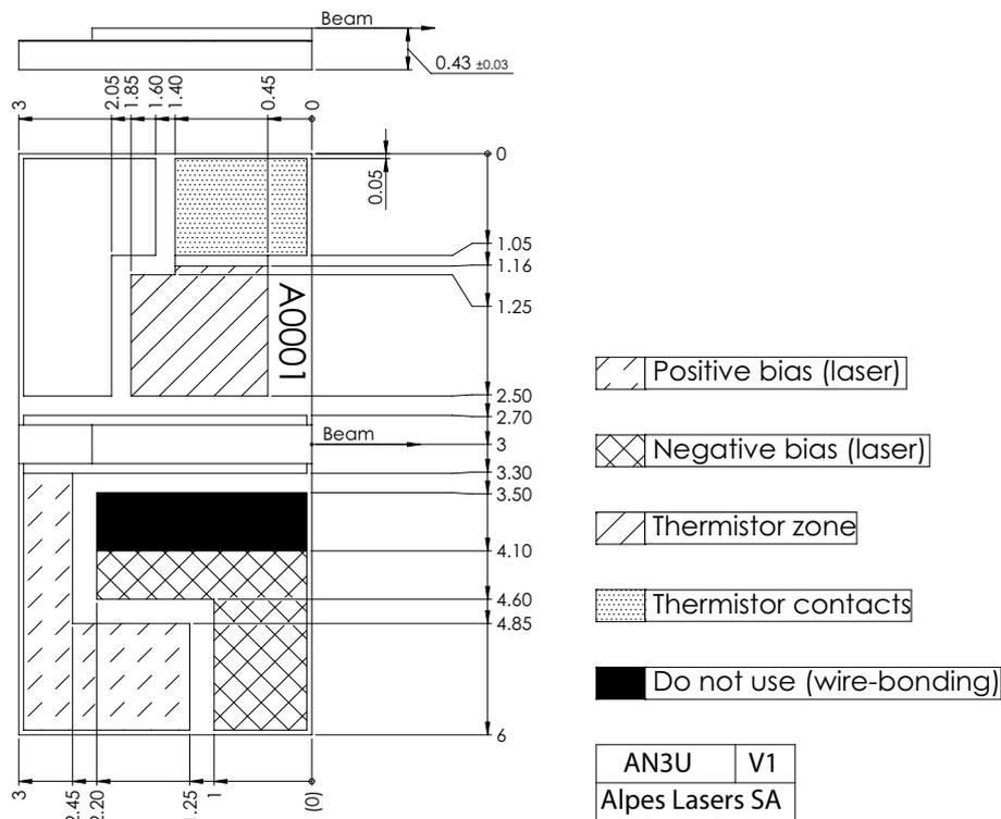
Figure 1: Mechanical and electrical interface for #sbcw20455 DN (please note that AlN submount numbering is A0RNT)
