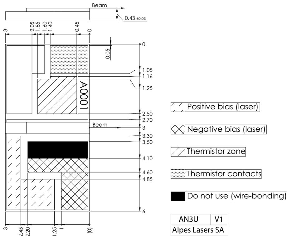
Figure 1: Mechanical and electrical interface for #sbcw21581 DN (please note that AlN submount numbering is A0NXX)
