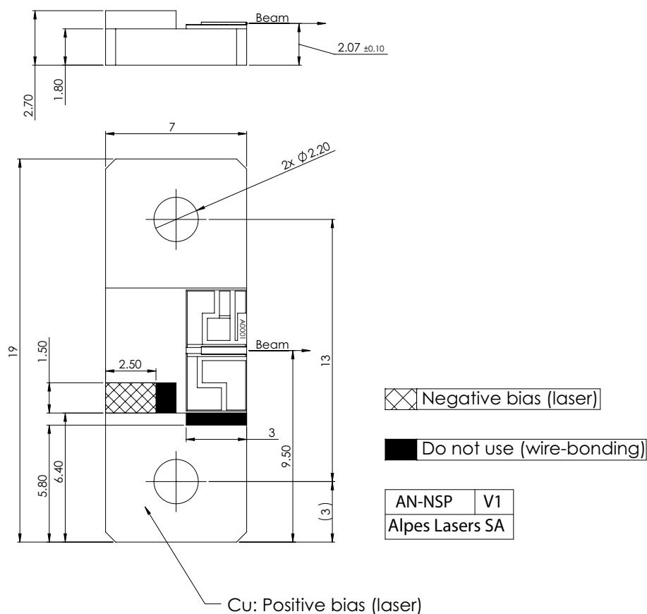
Figure 1: Support mounting for #sbcw6973 DN
