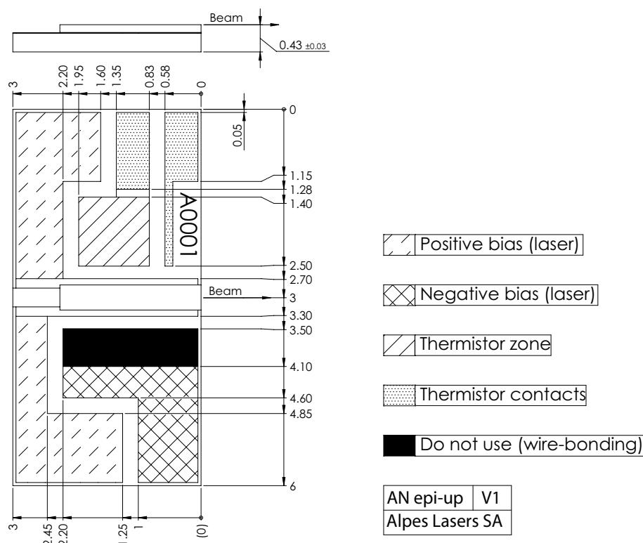
Figure 1: Support mounting for #sbcw8236 DN (please note that AlN submount numbering is A02A2)
