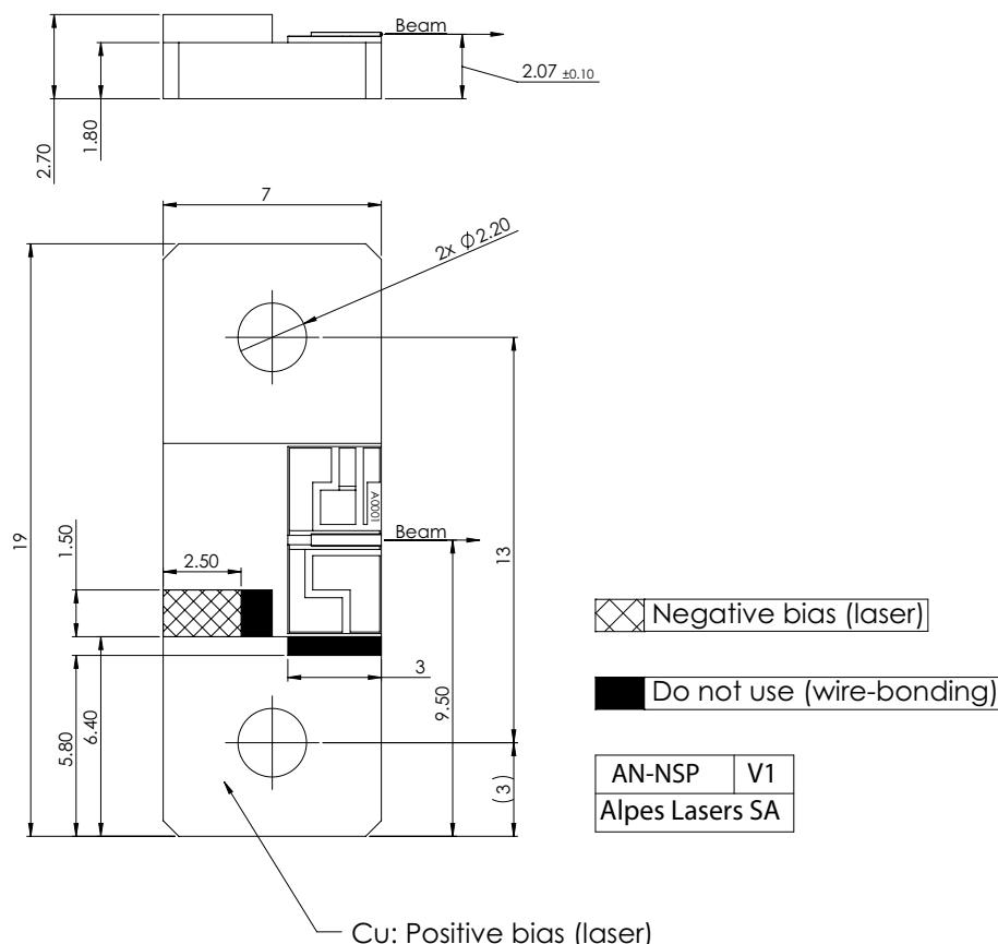
Figure 1: Mechanical and electrical interface for #sbcw8340 DN
