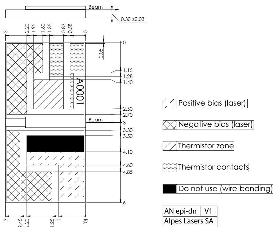
Figure 1: Mechanical and electrical interface for #sbcw8589 DN (please note that AlN submount numbering is A0054)
