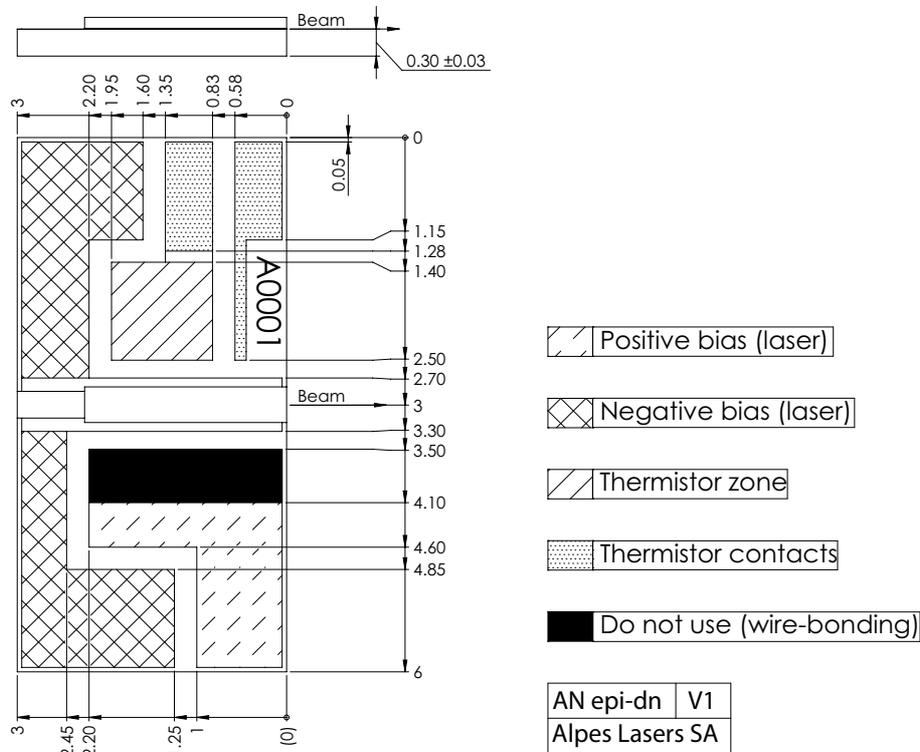
Figure 1: Support mounting for #sbcw8591 DN (please note that AlN submount numbering is A004C)
