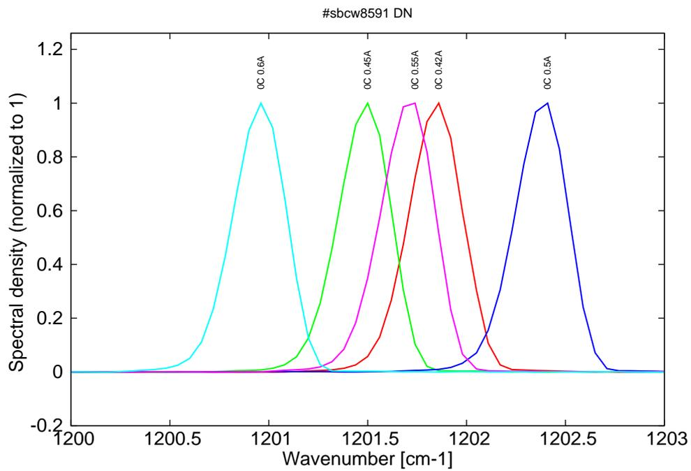
Figure 8: spectra at 0C for various DC currents (monomode on mode 1 up to 0.45A, then becomes monomode on mode 2, see Fig. 2 & 3)
