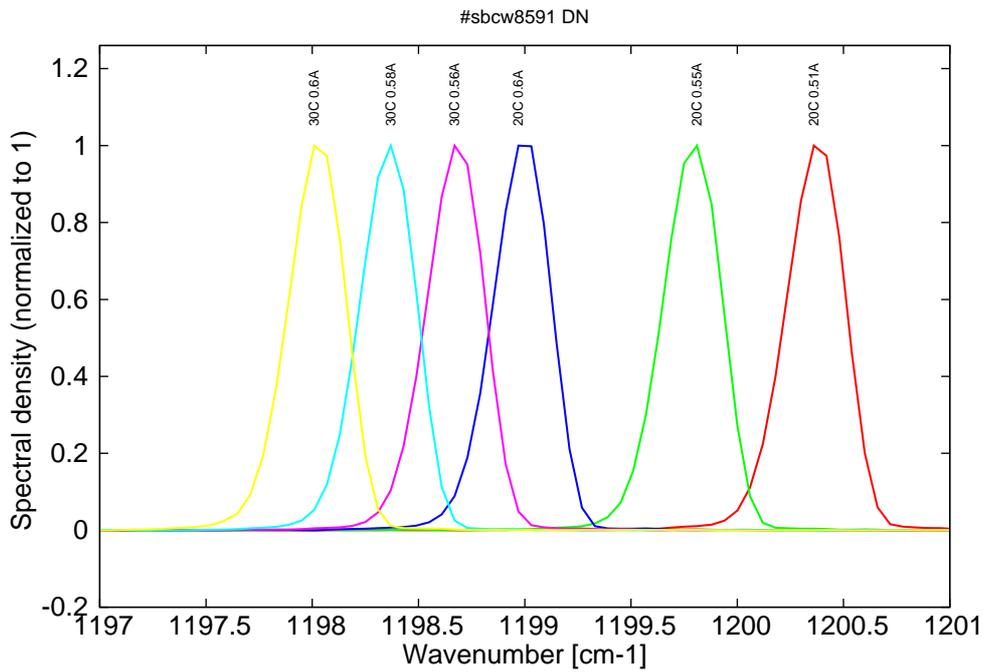
Figure 10: spectra between 20C and 30C for various DC currents (all monomode on mode 2, see Fig. 2 & 3)
