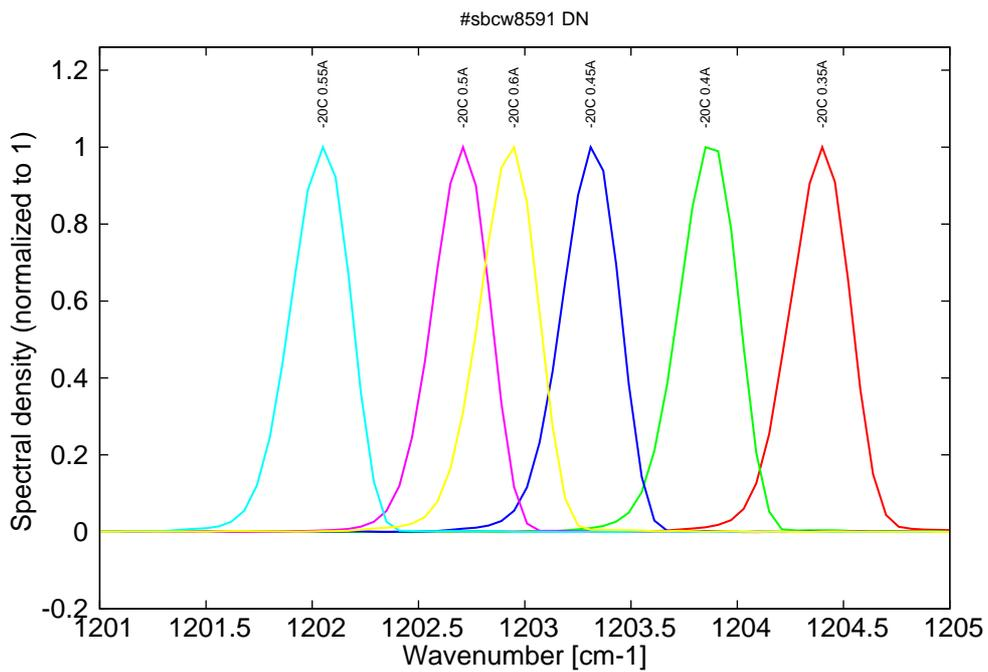
Figure 6: spectra at -20C for various DC currents (monomode on mode 1 up to 0.55A, then becomes monomode on mode 2, see Fig. 2 & 3)
