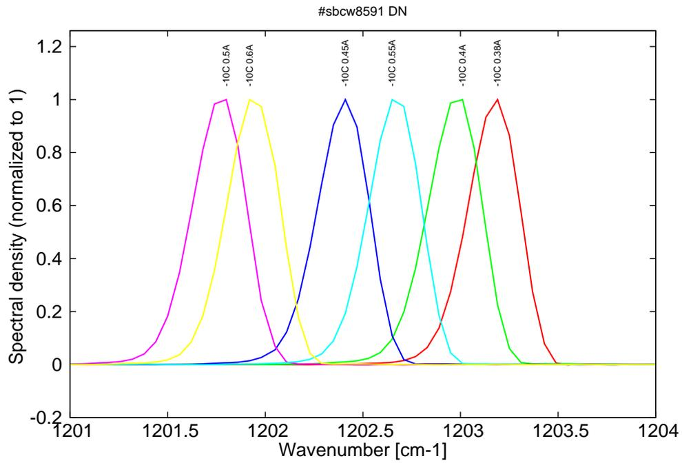
Figure 7: spectra at -10C for various DC currents (monomode on mode 1 up to 0.5A, then becomes monomode on mode 2, see Fig. 2 & 3)
