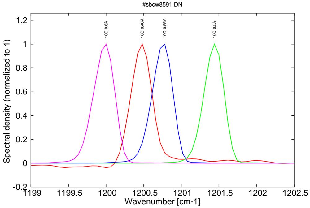
Figure 9: spectra at 10C for various DC currents (monomode on mode 1 up to 0.45A, then becomes monomode on mode 2, see Fig. 2 & 3)
