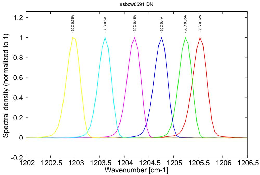
Figure 5: spectra at -30C for various DC currents (monomode on mode 1 up to 0.55A)
