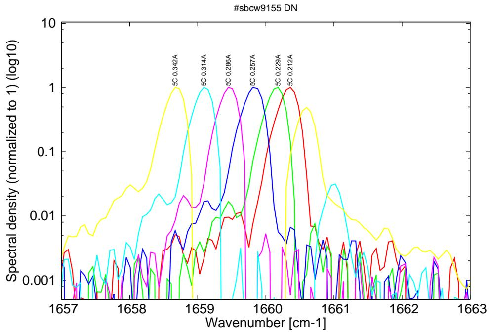
Figure 8: spectra at 5C for various DC currents (monomode up to 0.285A, then bimode)
