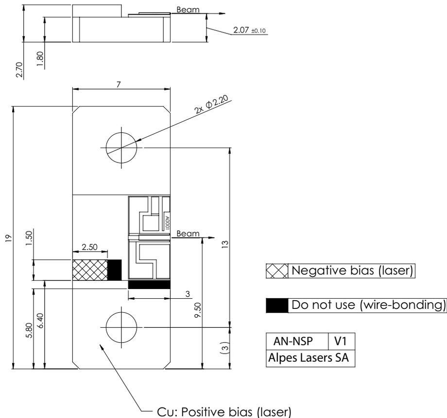
Figure 1: Support mounting for #sbcw9155 DN
