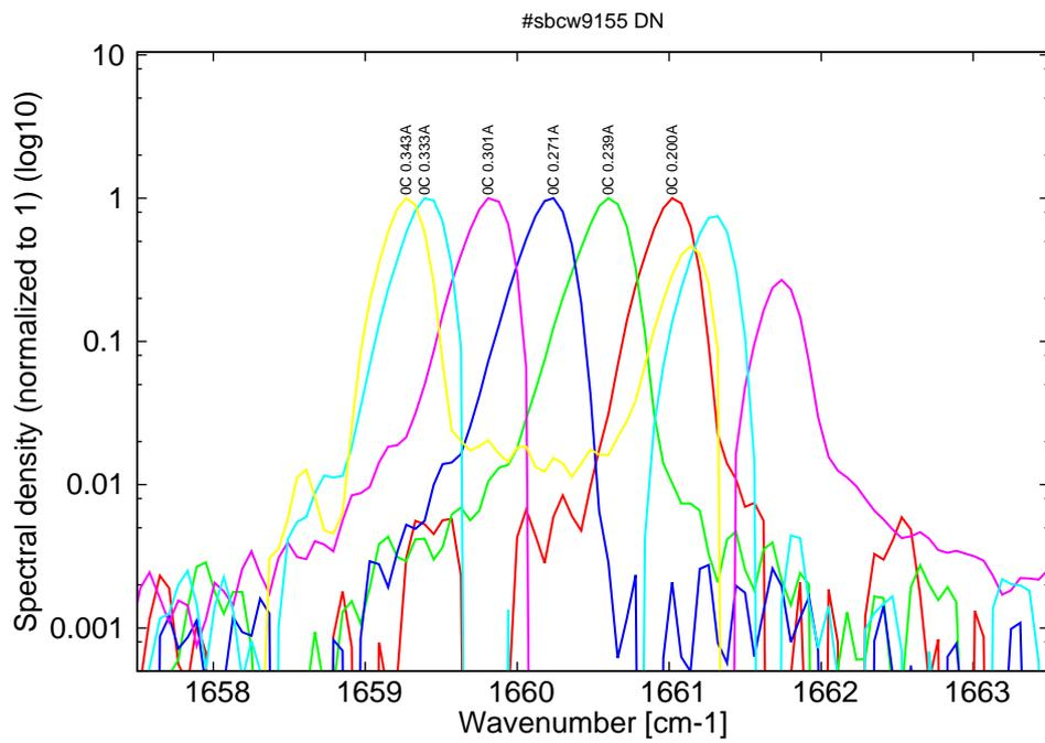
Figure 7: spectra at 0C for various DC currents (monomode up to 0.27A, then bimode)
