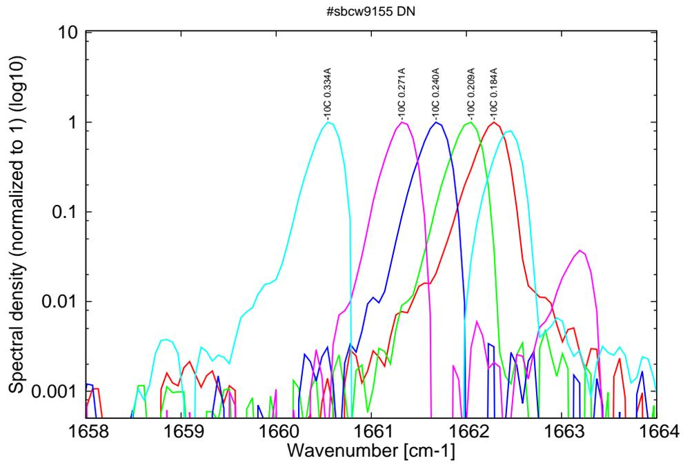
Figure 6: spectra at -10C for various DC currents (monomode up to 0.24A, then bimode)
