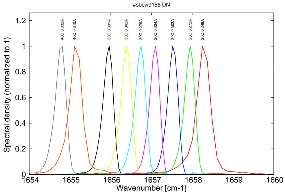
Figure 10: spectra at between 20C and 40C for various DC currents (monomode up to 0.335A)
