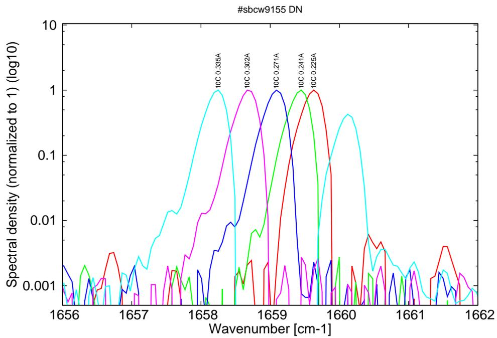
Figure 9: spectra at 10C for various DC currents (monomode up to 0.30A, then bimode)
