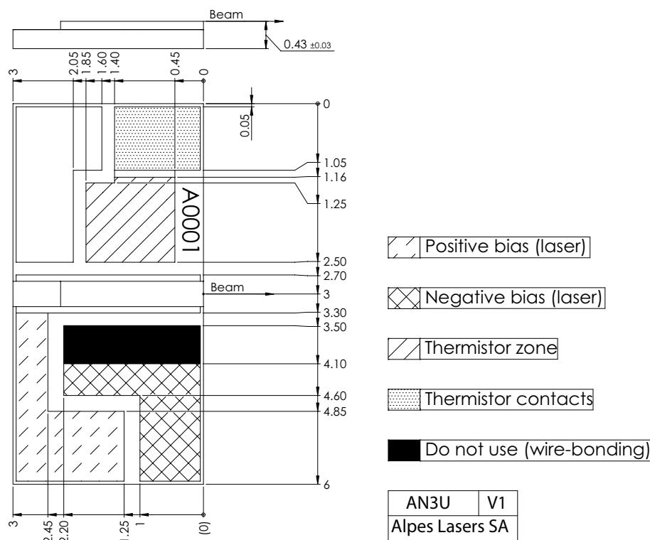
Figure 1: Support mounting for #sbcw9179 DN (please note that AlN submount numbering is A00UN)
